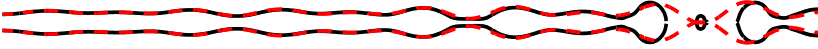
Figure 6.3: Superposition of two Rayleigh-Plateau-unstable modes on a liquid jet. The linear approximation (dashed line) and the numerical simulation (solid line) agree very well, until the satellite droplets start to form. The Weber number of this jet is 300, the value of n = 2 . This figure shows that linear superposition of the two perturbations gives a good approximation when the perturbation amplitude is small.
